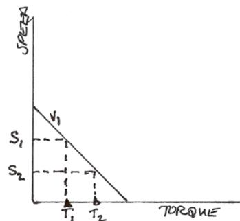
Figure 3 Speed-torque characteristic
