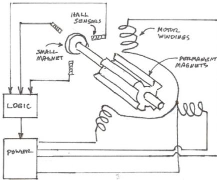
Figure 2 Electronic commutation of brushless motors
