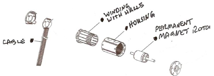
Actually, the brushless motor has no part in "commutation" it is accomplished by the control, that is supplying power running the motor, which accomplishes the "electronic commutation". Figure 2 illustrates the concept of how electronic commutation works. For this example, the brushless motor consists of a rotor with permanent magnets, stator with windings and a small feedback device (that consists of a small magnet and three Hall sensors).
