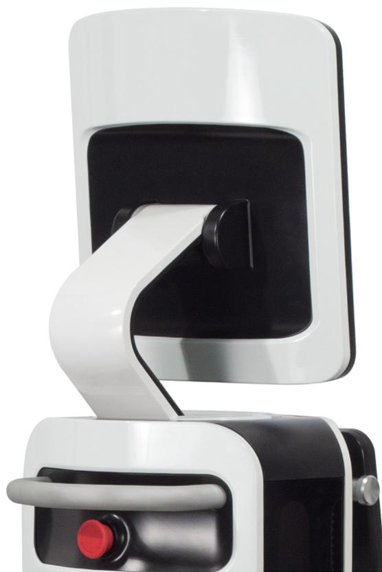
**Figure 3:** The display/camera module of RP-Vita features tilt capabilities where the "neck" attaches to the display and pan capabilities in the "shoulder" region where the neck attaches to the torso. (Courtesy of InTouch Health)
