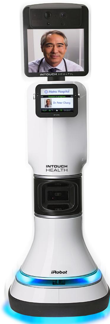
**Figure 2:** The anthropomorphic unit consists of a 49-in. torso topped by a display that integrates embedded high-resolution cameras with pan-tilt capabilities. (Courtesy of InTouch Health)
