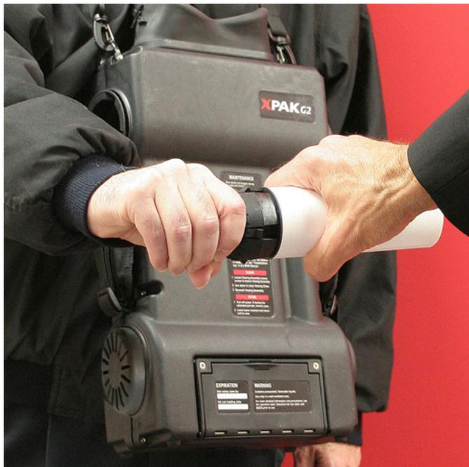
**Figure 2:** Measurements start by wiping a removable baton wrapped with specially treated paper against the target of interest. (Courtesy of RedXDefense)
