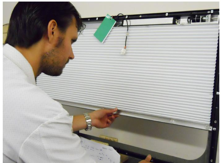
asked me to put it in what's referred to as an out-of-plane configuration, where the shade is bent. [The gearmotor] made it to 235,000 cycles and it was still running when we stopped it."
