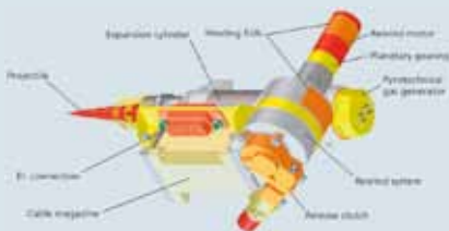
Design configuration of the "harpoon anchor"
